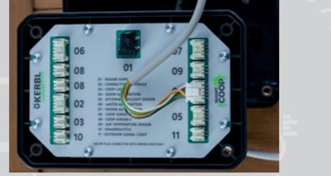
If the connection cable built into the module is not long enough, it can be lengthened using extension cables (items 70633, 70634). Ensure that the connection location is protected from water and dust. The module cable must have only a single extension.
